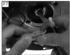
Connect plug from fan to switch house plug.
